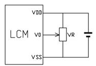
V<sub>DD~</sub>V<sub>0</sub>: LCD Driving voltage VR: 10k~20k
